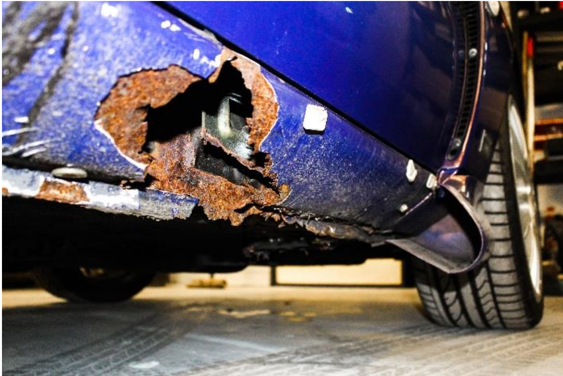
Sills rusted through underneath body kit, also eating into the edge of the floor
