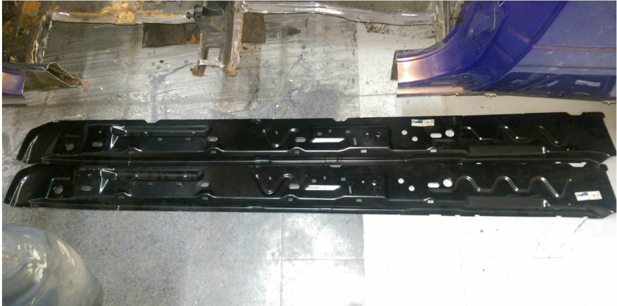
New sills had to be sourced from America as there were none available in Europe
