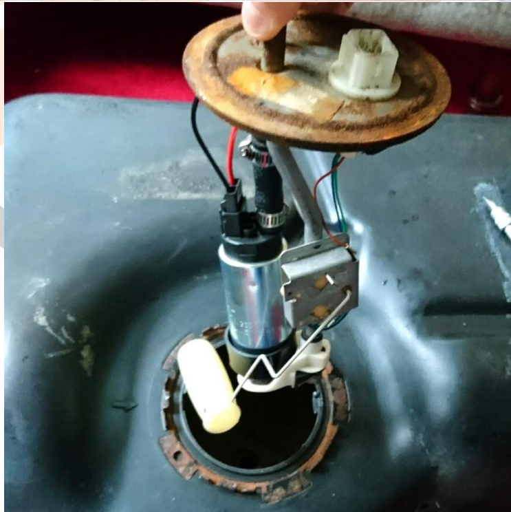
Fuel pump replacement
