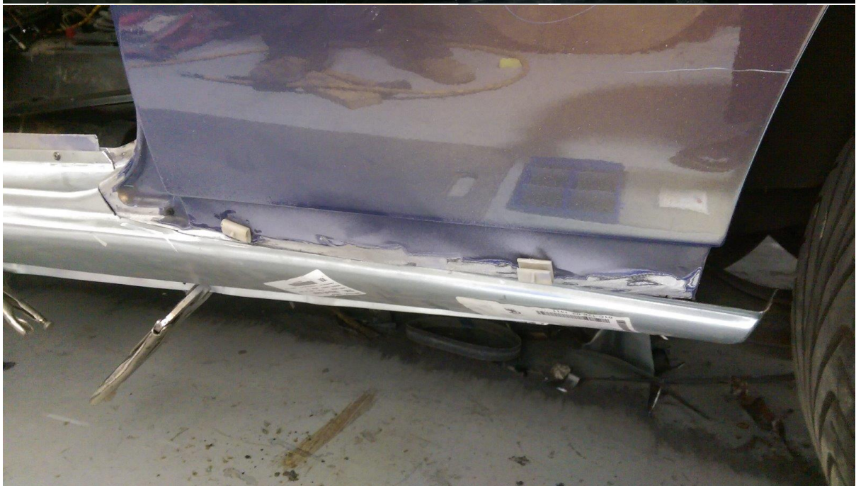
New outer sill measured for cutting and fitting
